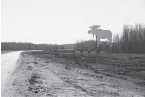
**Figure 25.** Specialized signage, such as this one near Grand Prairie Alberta can be used to alert drivers to areas of recurrent Moose-vehicle collisions. Changing signs regularly and placing them in seasonally relevant places along the highways inhibits desensitization of motorists to wildlife warning signage. 16 April 2006 (Roy V. Rea).
